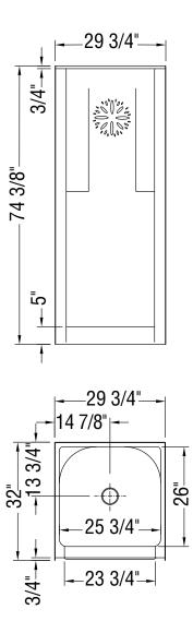
All dimensions are approximate. Structure measurements must be verified against the unit to ensure proper fit.
