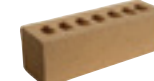
Metric Jumbo Length 290 mm (11 1/2") Height 90 mm (3 1/2") Depth 90 mm (3 1/2") Bricks per square foot 3 Bricks per square metre 33
