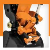
■ Manual wedge-style coupler enables quick changes and a wide variety of buckets and attachments, such as breakers and augers.
