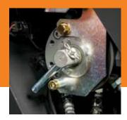
■ Go from backhoe- to excavator-style controls with just a twist of your wrist. Control-pattern selector valve is conveniently located in a compartment beneath the seat and includes a sight glass that displays the selected pattern.
